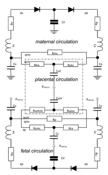
Figure 2: Electrical analog of blood flood system in the model. [3]
